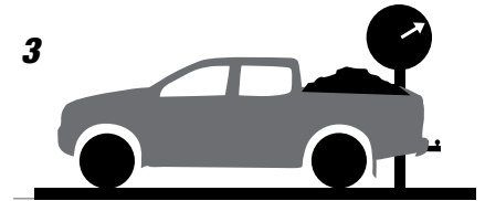
3 1 + 2 = Total weight of vehicle Ensure total weight does not exceed manufacturers GVM (gross vehicle mass)
