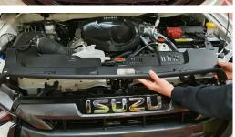
STEP 2 Remove slam panel cover and set to one side.
